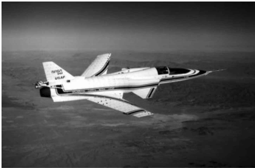
Dryden Flight Research Center EC90-039-4 Photographed 1990 X-29 at an angle that highlights the forward swept wings. NASA photo by Larry Sammons
